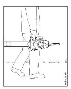
It may be carried only in the horizontal position. Grip the front handle and keep the hot muffler away from your body and the cutter blades behind you.
