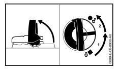
Flip up the lever and slowly turn left (1) to the vent position of the cap at about 1/8 turn where the cap is held in place by the thread. Once the fumes have been relieved, turn (2) the cap further to the 1/4 turn position where the tool-less cap can be removed from the tank thread.
