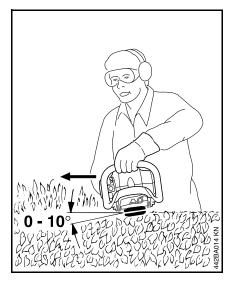
Hold the cutter bar at an angle of  $0^{\circ}$  to  $10^{\circ}$  as you swing the hedge trimmer horizontally.
